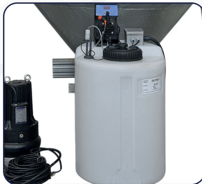
Automatic flocculant dosing station: Adds flocculant in a controlled manner to enhance settling and sedimentation of solids.
