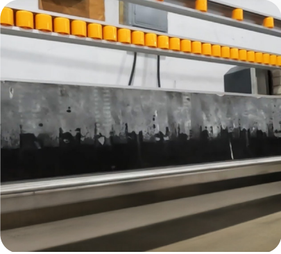
Left-hand output arm: System that delivers the part already polished.
